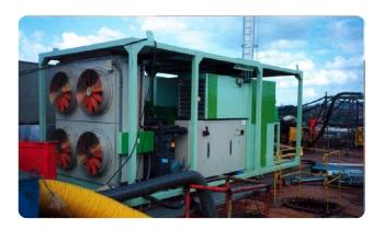
By way of example, FISAIR supplied 12 DFRC-2100-E and 4 DFRC-1300-E units, all with a cooling system, for temperature and humidity control inside the tanks of the ships, during the interior coating of these.
