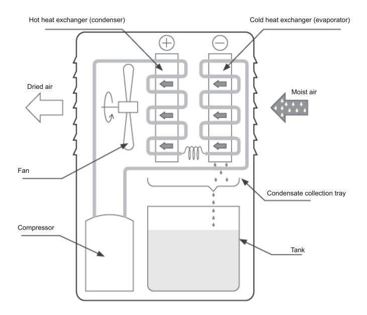
When the dehumidifier operates with an internal tank the dehumidifier will switch off when the tank is filled with condensate. The tank filling indicator «FULL» lights up on the control panel display. For the dehumidifier further operation it is required to remove the internal tank, to release it from water and to install back into the humidifier . «FULL» indicator will go down.
