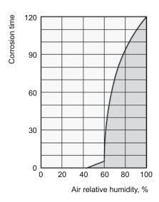
As you can see, the rate of corrosion is insignificant at the relative humidity below 50%, and it can be disregarded at the relative humidity below 40%. But at the relative humidity above 60% the rate of corrosion increases considerably.
